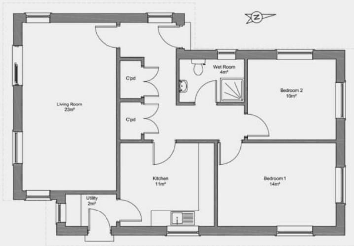
Proposed Floor Plan - 1:50 Gross External Area = 95m 2
