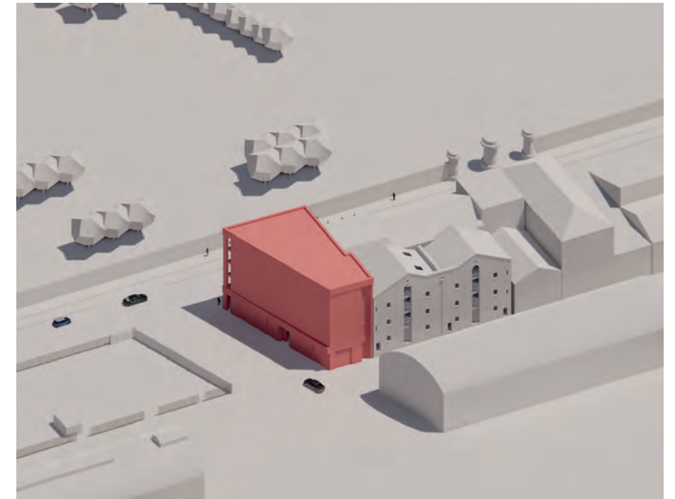
A plinth level was established to further emphasise this layering along with a setback to the upper floors reducing the proposal.
